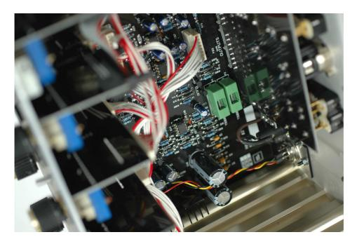
IC sockets, together with additional power decoupling were fitted to enable a wide range of opamps to be tried. Eventually a combination of Burr Brown and National Semiconductor opamps was settled upon.
