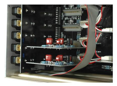
Op-amp replacement was the next procedure. No one we spoke with had replaced op-amps on an LE edition before. Simply swapping out docile TLO72s with high bandwidth modern op-amps is a risky procedure, as one does not know if power bypassing and the PCB layout are up to scratch, potentially creating ultrasonic oscillation. The removal of the op-amps was performed with a temperature-controlled rework station. Care and patience had to be applied to ensure no damage to the PCB resulted.
