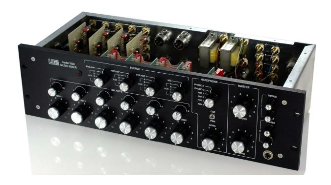
The headphone cue select switch was replaced with an ELMA type, famous for their use in EMI and Neve consoles. Tone bypass switches were added via a custom-made bracket. All additional was wiring performed with silver-plated / PTFE-insulated type, in keeping with its original use in the 1620:
