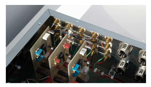
After this photo was taken, the preamp cards were fitted with precision 1% tolerance polypropylene foil / film RIAA capacitors.
